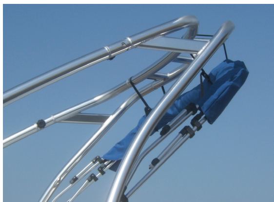
Convenient storage design allows top to be secured to the tower when folded back and not in use.
