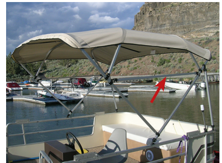
Free Standing Pontoon Bimini Top has a center cross strut for stability rather than front hold-down straps.
